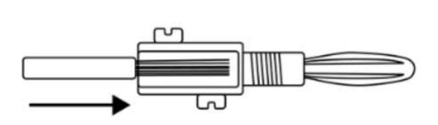
Strip wire 14 mm then insert wire into Banana Plug
