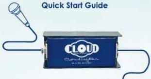
1. Connect the output of the Cloudlifter to a preamplifier, mixing console, audio interface, or any other source capable of supplying +48v phantom power. When using long cable runs, the Cloudlifter can be nearer the mic or the preamp, depending on the equipment used. Visit our website to learn mare.
